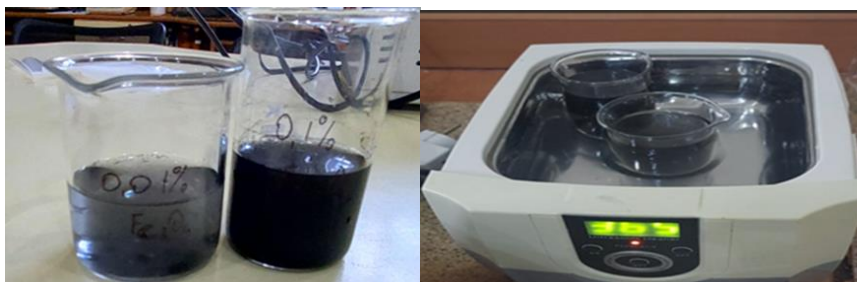
Figure 1. The preparation of the solutions of \text{Fe}_3\text{O}_4 nanoparticles.
